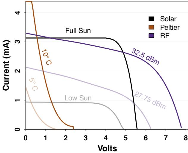
Figure 2. Six I-V curves are shown, produced by three different energy harvesters—a solar panel, a Peltier generator, and an RF Reader—each under two (2) different energy harvesting conditions. Each harvester produces its own “family” of curves, with a common characteristic shape. Each of the above I-V curves were captured with the recording feature of Ekho. Note that the Peltier curve has been scaled 17x for purposes of illustration.
