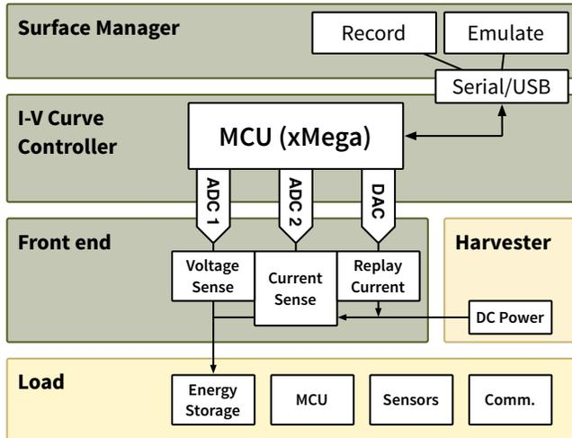
**Figure 6.** Ekho consists of three interdependent modules: a surface manager that stores I–V surfaces and manages the high-level recording and emulation logic for the system; a low-latency controller that sequentially emulates the I–V curves that correspond to each single point in time during an emulated surface; and a front-end module that facilitates controllable current emulation and provides signal conditioning that is needed for taking accurate current and voltage measurements.
