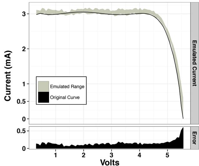
**Figure 13.** Shown in the top part of this figure are the target curve Ekho is emulating, and the actual range emulated for a number of test runs on a program. The bottom part of the figure shows the error amount for different parts of the emulated curve. As the slope increases, the current error increases past the knee of the I-V-curve.
