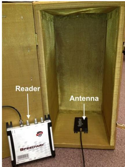
**Figure 12.** Our prototype RF-box provides a reproducible RF harvesting environment used in our experiments to provide “ground truth” harvesting conditions. The RF-box is composed of a wooden shell layered with brass screen copper mesh seals. Inside the box is an antenna, driven by a programmatically controlled reader.
