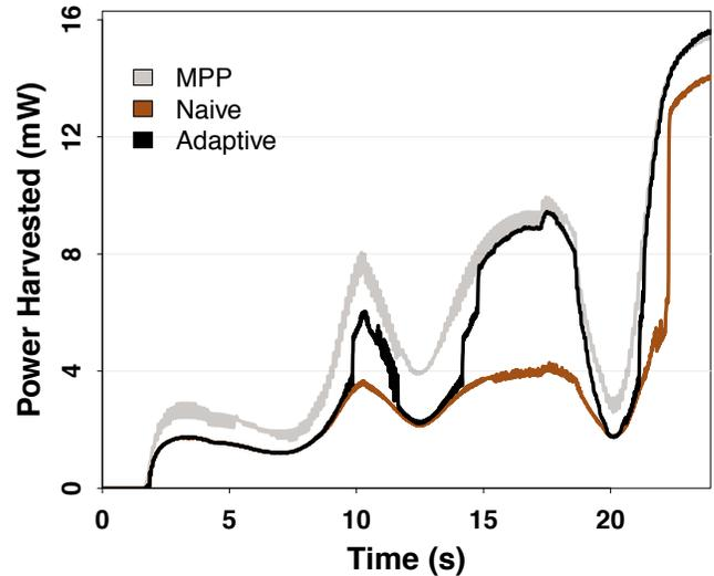
**Figure 1. Harvested power is shown for two TI EZ430-RF2500 target boards running different programs that both write to flash in different ways—one writes as fast as possible if there is any power available, the other adapts so it can write even when harvestable energy is scarce—under the same solar energy harvesting conditions. Differences in power consumption result in different amounts of harvested power.**
