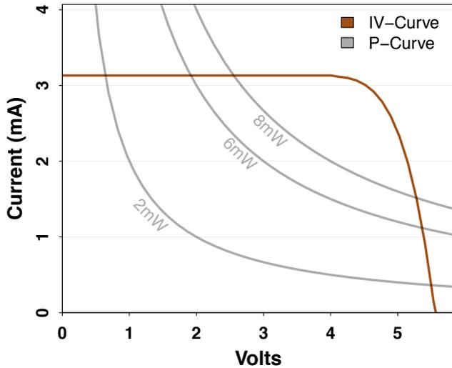
Figure 4. Shown is a single I-V-curve, and the consequences of choosing constant power to represent it. Depending on the load, the generated P-curves from the power trace can cause unrealistic changes in the programs actual harvested energy. As shown, emulating constant power is a poor replacement for emulating the actual I-V-curve.
