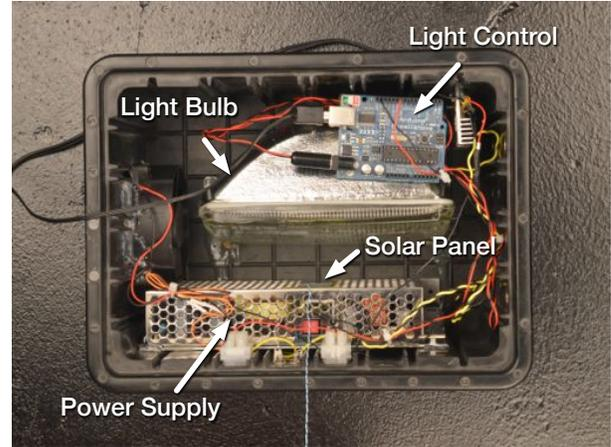
**Figure 11.** Our prototype light-box implementation provides a reproducible solar harvesting environment that we use in our experiments to provide reproducible “ground truth” harvesting conditions. The implementation consists of a automotive headlight, a solar panel, an Arduino which serves as programmable dimmer-switch, and necessary power supply.
