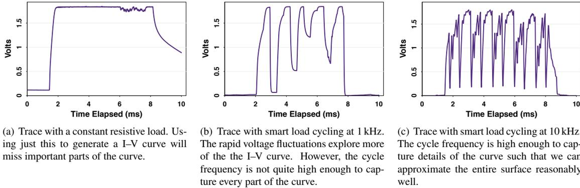
**Figure 8. RF energy harvesting voltage trace over 10ms, with three different custom “smart” load cycle frequencies.**
