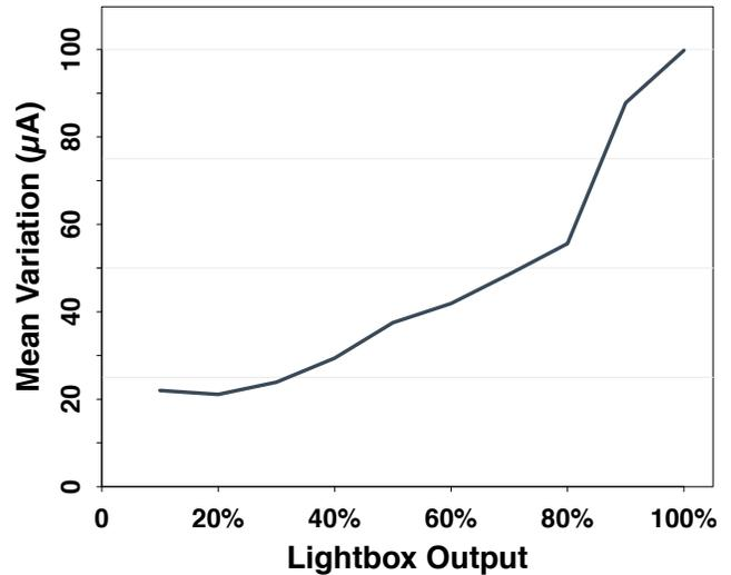
Figure 5. The light-box mean variation between runs increases with light intensity for static loads. The light-box, unlike Ekho is susceptible to environmental changes and care must be taken to control those. Temperature changes after long use are one such factor that affects repeatability.
