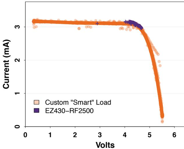
**Figure 7.** This figure shows recorded I-V measurements, as produced by both the Ekho smart load device and a typical mote-class sensor device. By intentionally increasing the power supply volatility, the smart load provides much better coverage of the I-V curve being recorded, which improves Ekho’s recording accuracy.
